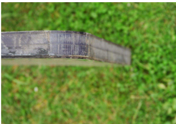
ARMoured GLASS - 42MM THICK! ITS BULLET PROOF, TOO.
