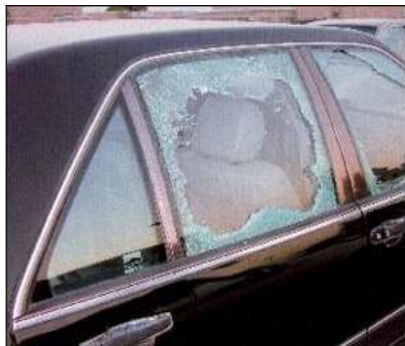
THE OUTER SHEET OF GLASS IS BROKEN BUT THE INNER LAYER IS STILL INTACT.
